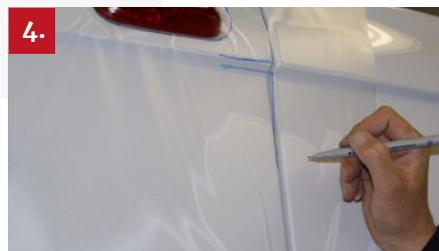
5 Vinyl kits should conform to any external 2D radius; however, as these materials are non-conformable to recesses and complex curves, please mark clearly any recesses and complex curves on the template so that the appropriate chevron pieces can be supplied.
