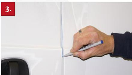
4 Mark around any area which has a recess, marking both internal and external folds.
